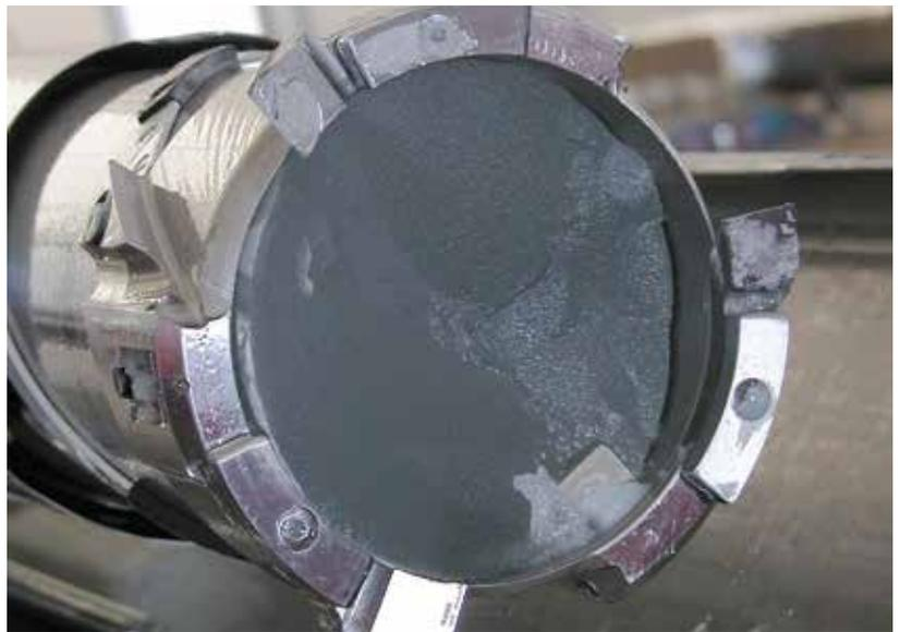
Drill head of the EPICA drill used at Dome C (Antarctic) containing a 10 cm diameter ice core
