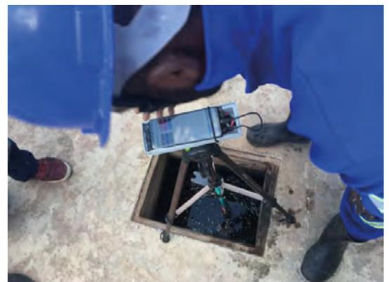
Using the Volaser with the smartphone app in a septic tank in Lusaka, Zambia. © Eawag
