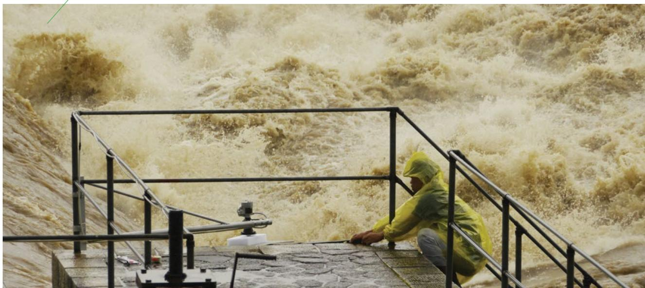
*Technician testing a radar water level sensor in an early warning system supported by GIZ in Phu Yen province\_Edit*
