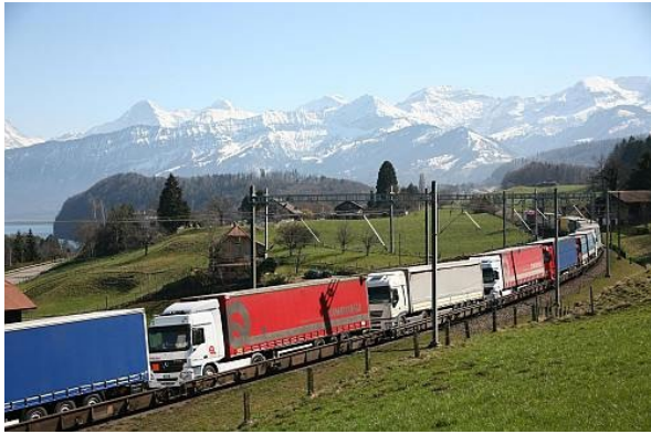
72% of freight crossing the Alps now goes by rail using systems like the 'Rolling Highway', where entire trucks are loaded onto trains © International Railway Journal
